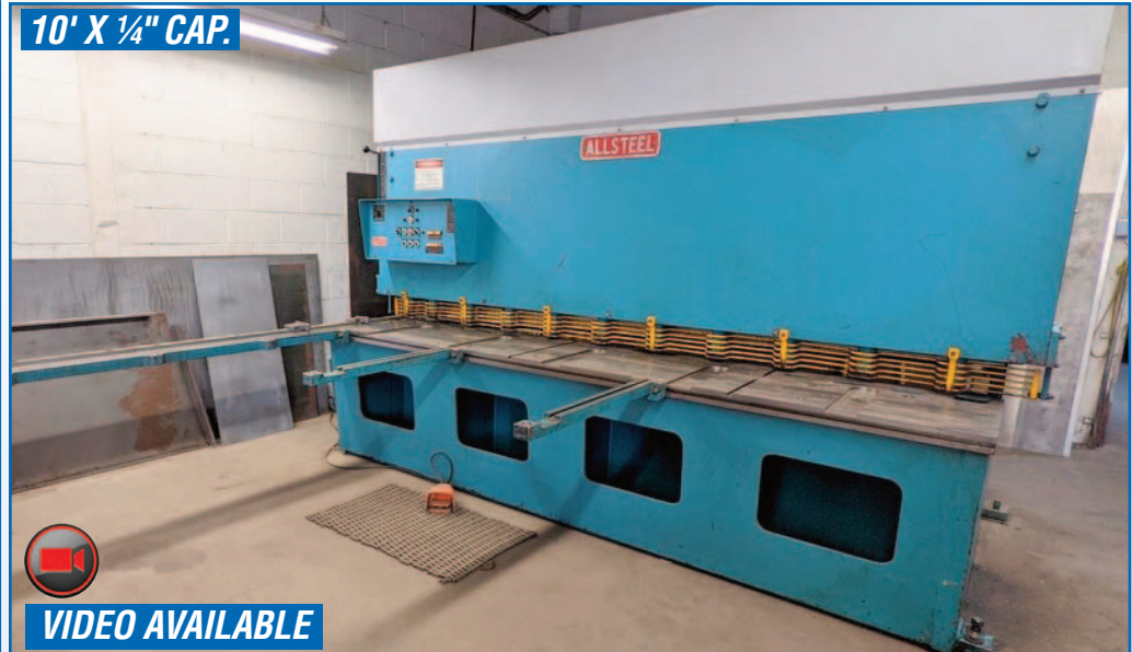
ALLSTEEL 1/4-10 HYDRAULIC POWER SQUARING SHEAR
